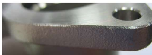
Detail view: flange deburred with engraflexx
